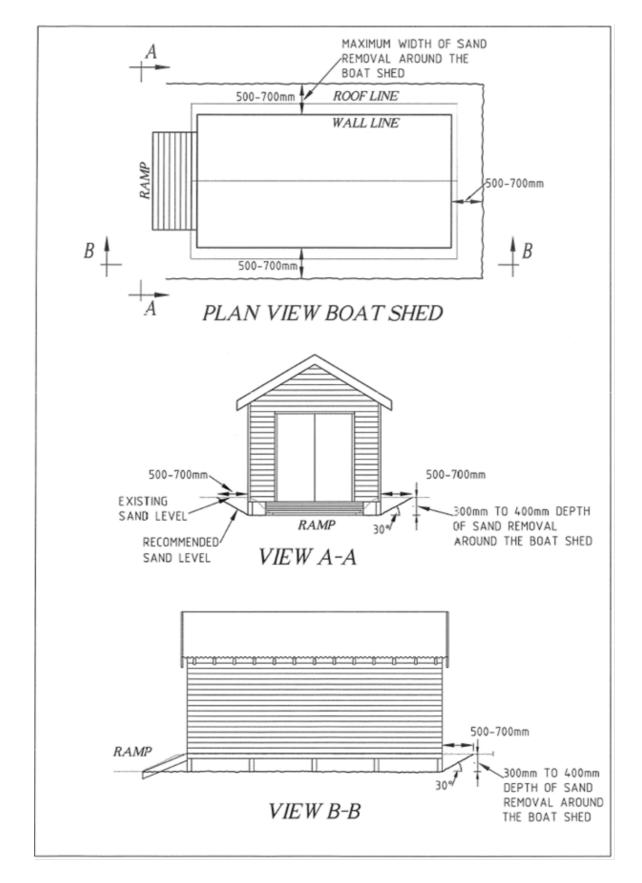
Plan showing clearance of sand around Boatshed/Bathing Box at 30-degree horizontal fall.
