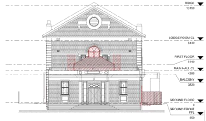
EXISTING SOUTH-WEST ELEVATION SCALE 1:100
