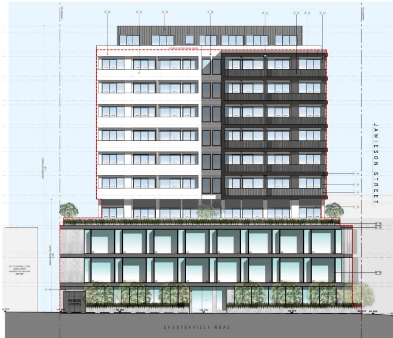
Image 6: Proposed eastern (Chesterville Road) elevation with the approved ten storey building shown by the dashed red line.
