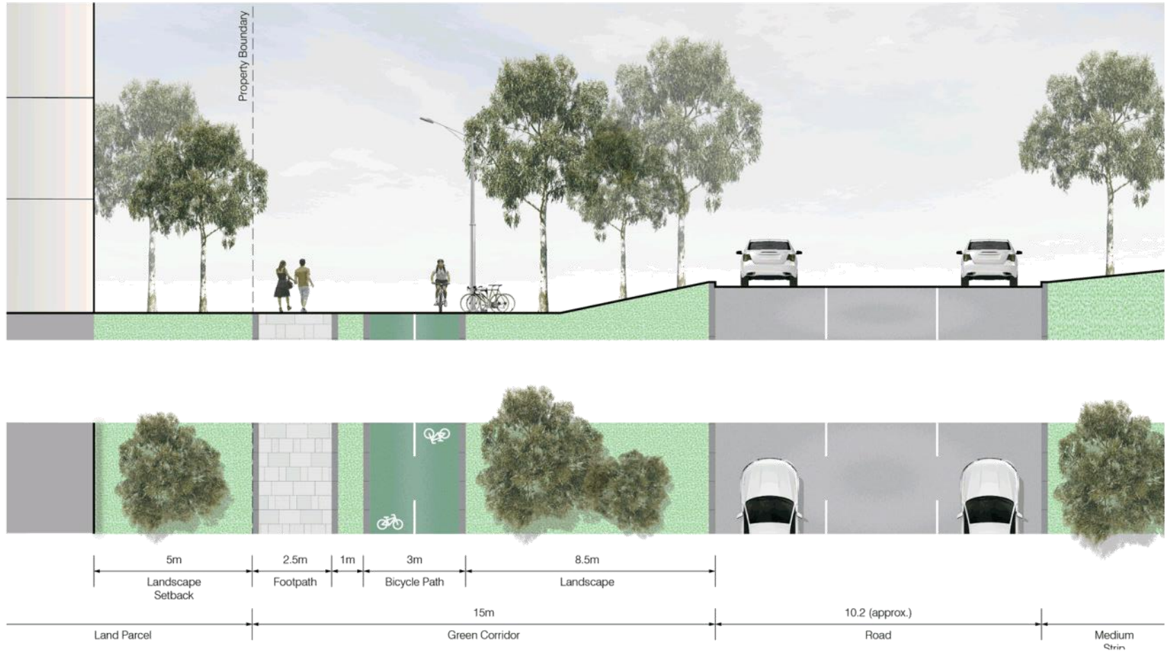
Figure 14: Nepean Highway Interface Section
