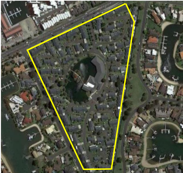
Figure 8. This image presents a notable hot area in the landscape, showing dark roofed buildings and small-medium sized blocks with the total impervious area taking up a large proportion of the block.
