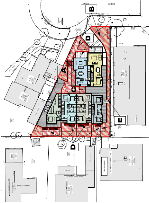
DESIGN RESPONSE - FIRST FLOOR PLAN 1:200 @ A1 *garden area shown in red diagonal hatch pattern = 253m 2
